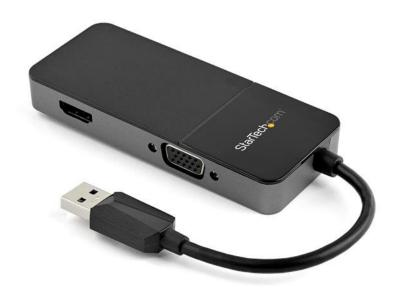
This USB 3.0 to HDMI VGA adapter offers a portable solution for connecting an HDMI and VGA display to your USB-A laptop or desktop computer. The multiport video adapter lets you mirror or extend content on two additional monitors simultaneously (1  $\times$  HDMI and 1  $\times$  VGA), creating a dual-screen workstation. The adapter is backward compatible with USB 2.0 computers (optimal performance with USB 3.0, backward compatible with USB 2.0).
