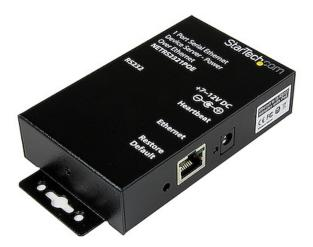
The NETRS2321POE 1 Port RS232 Serial Ethernet Device Server - PoE (Power Over Ethernet) allows you to install your RS232 devices anywhere on your TCP/IP Ethernet WAN/LAN, and access them as if they were right beside you - even over the Internet!
