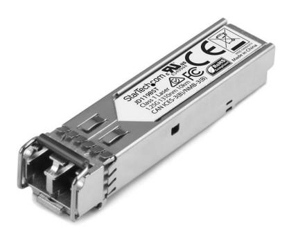
The JD119BST is an HP JD119B compatible fiber transceiver module that has been designed, programmed and tested to work with HP® brand switches and routers. It delivers dependable 10 GbE connectivity over fiber cable, for 1000BASE-LX compliant networks, with a maximum distance of up to 10 km (6.2 mi).
