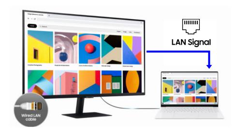
If your laptop does not have a LAN port, you can still use an Ethernet connection by connecting the wired LAN port directly to the monitor. This transmits the LAN signal to the connected laptop.
