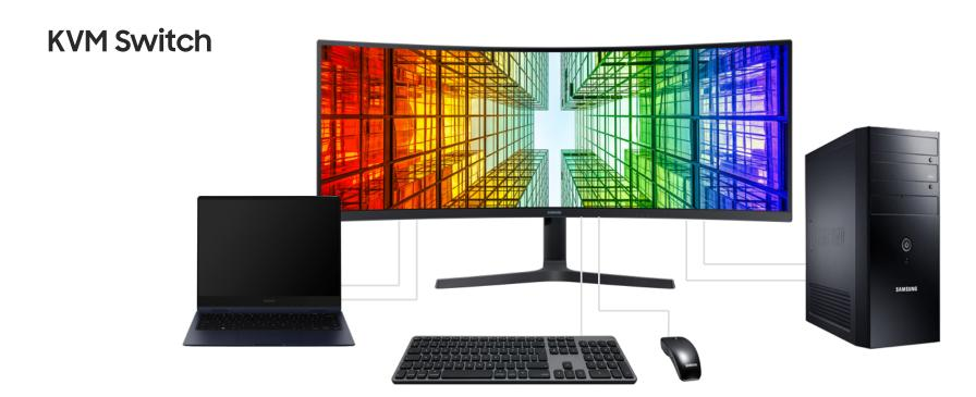
A built-in KVM switch allows the user to control two sources connected to the monitor, with just one keyboard and mouse. Once connected, users can effortlessly toggle between sources using the one-touch button on the monitor's bottom bezel, removing any multi-device hassle and enhancing efficiency.
