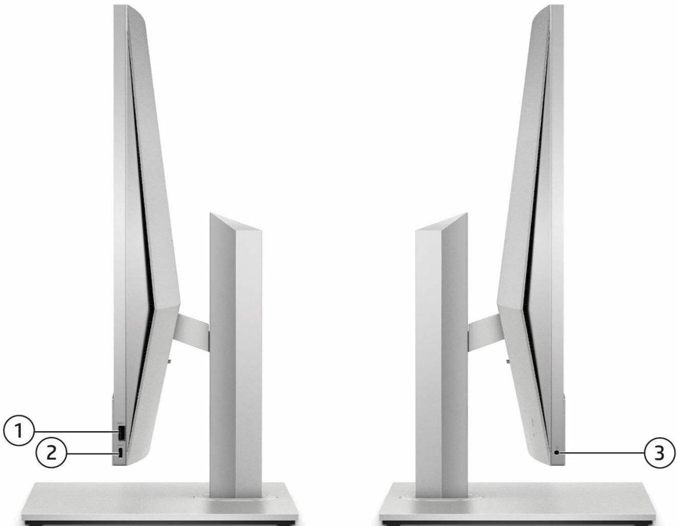
1. Type-A SuperSpeed USB 10Gbps signaling rate port (charge support up to 5V/3A)
