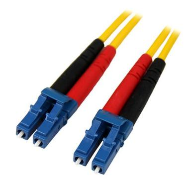
The SMFIBLCLC1 1m LC to LC Single-Mode Duplex Fiber Cable features 9/125 micron fiber for high-speed, high bandwidth data transmissions over Gigabit Ethernet and Fiber Channel networks, with support for duplex single-mode applications.
