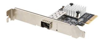
This PCIe network card lets you take advantage of improved bandwidth in data-intensive applications such as multimedia streaming and large file transfers. This fiber NIC offers data transfer rates of up to 10Gbps which improve speeds and reduces load times.
