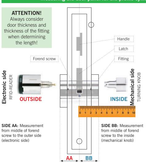
When determining the required cylinder length, the thickness of the fitting in use always has to be added to the door thickness. Always select the next higher measurement to what you measured in 5 mm increments. Beginning at the **basic** dimension of 30 mm for profile cylinders or 32 mm for Swiss round cylinders respectively per side (AA/BB), up until the maximum length of 70 mm or 72 mm respectively per side (AA/BB).
