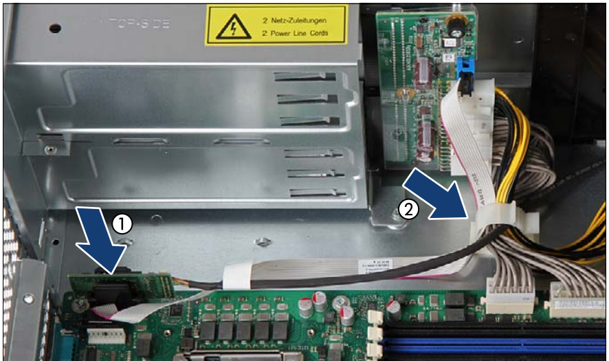
Figure 256: Connecting the front LAN board to the system board
