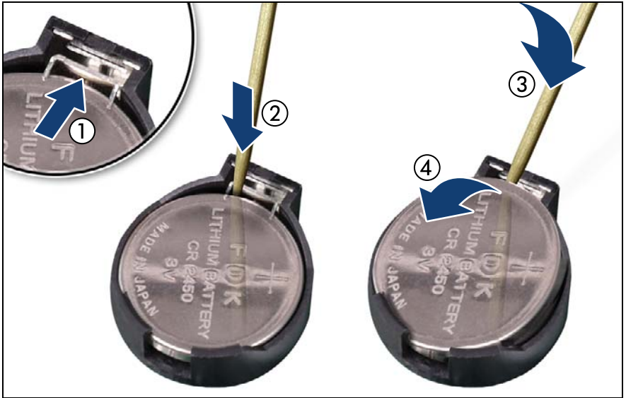
Figure 262: Replacing the CMOS battery
