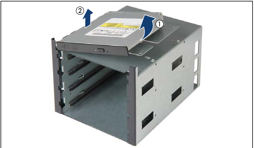
Figure 240: Removing the slimline ODD from the extension box (B)
