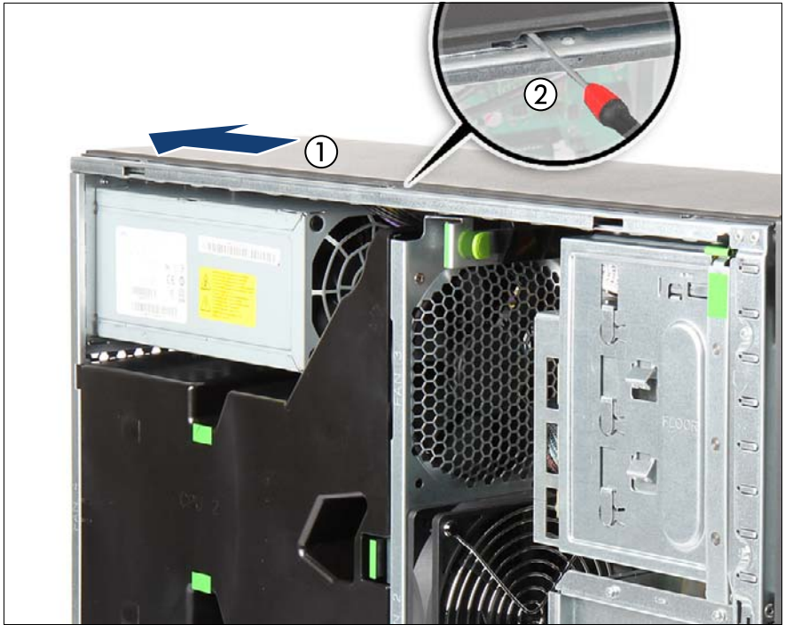
Figure 295: Removing the right side cover (B)
