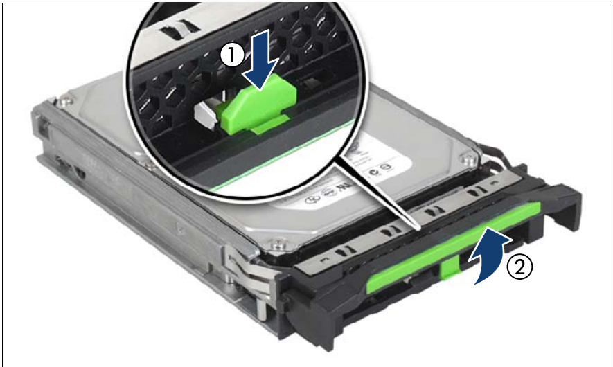
Figure 84: Opening the 3.5-inch HDD module locking lever
