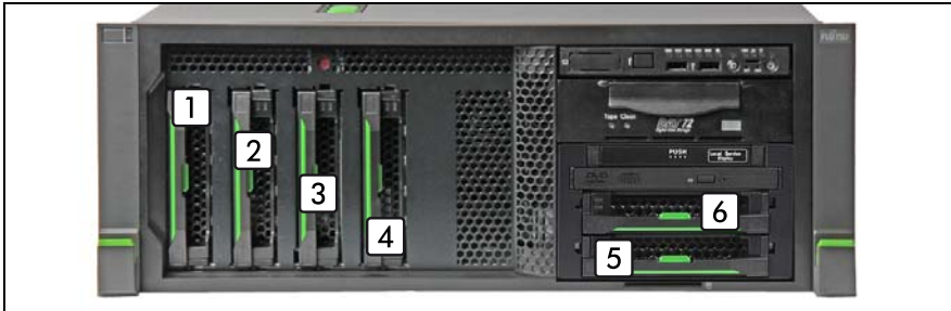
Figure 79: Naming scheme with 10 3.5-inch HDDs (2 SAS backplanes) - Rack version
