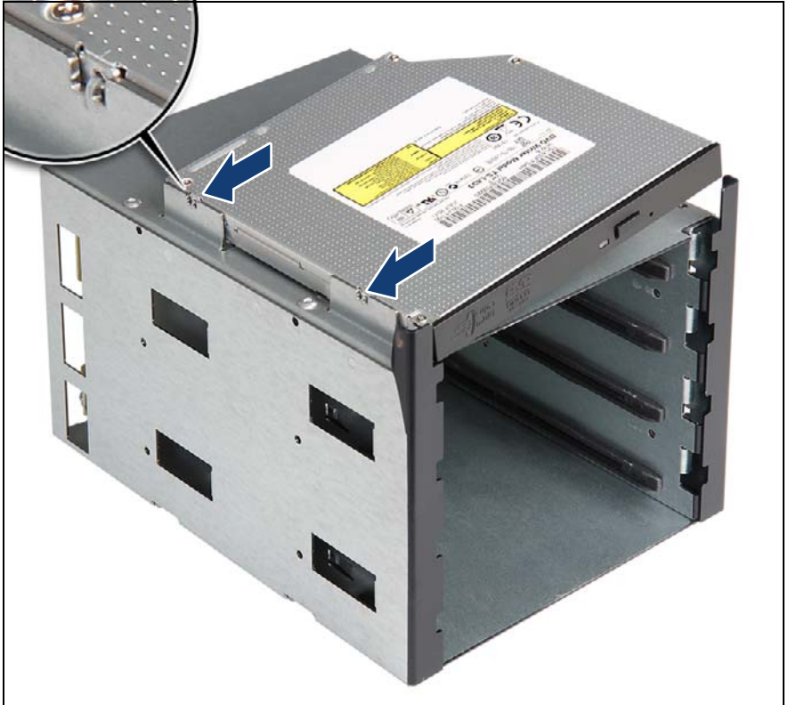
Figure 235: Installing the slimline ODD on the HDD extension box
