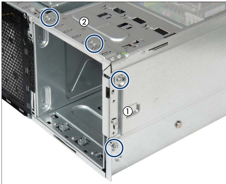
Figure 298: Detaching the accessible drive cage (B)
