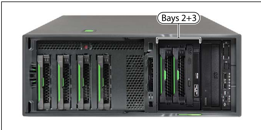
Figure 100: 2x 3.5-inch HDD extension box - Tower version
