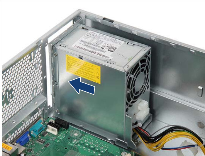
Figure 47: Installing PSU in the chassis (B)
