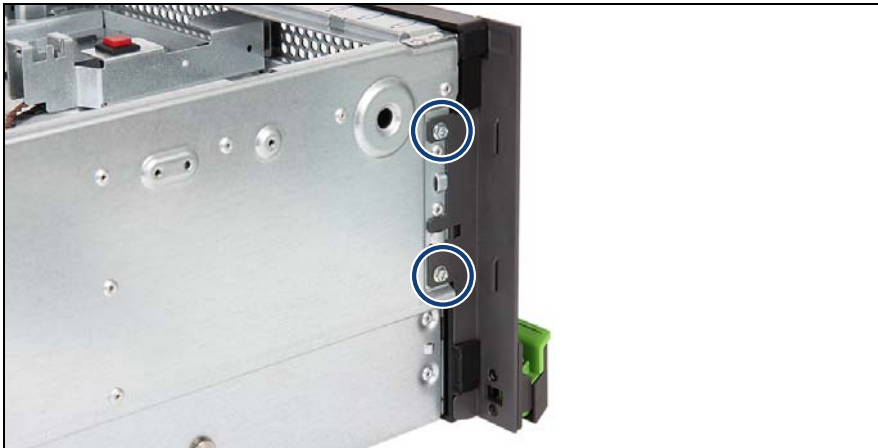
Figure 7: Removing the rack front cover (A)
