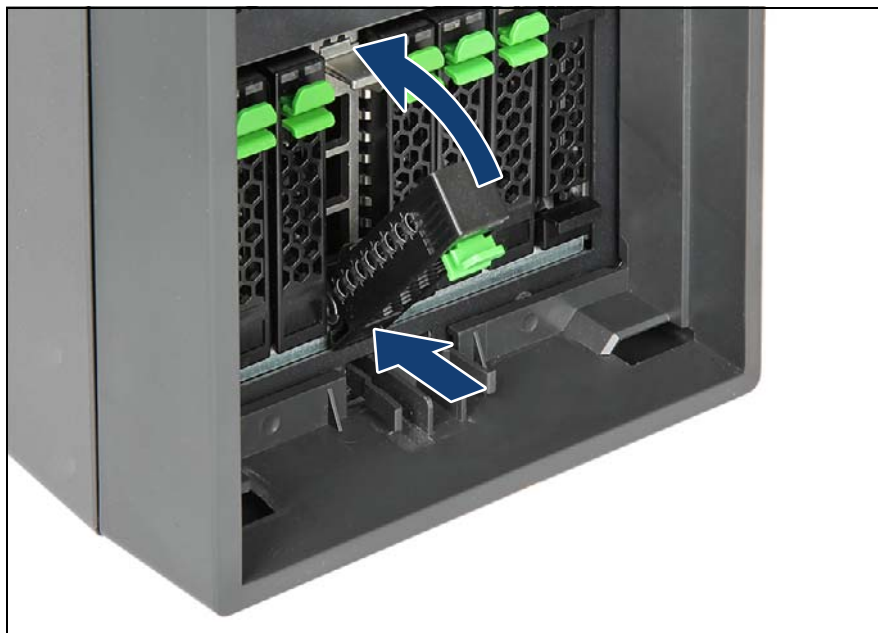
Figure 69: Inserting the 2.5-inch HDD / SSD module
