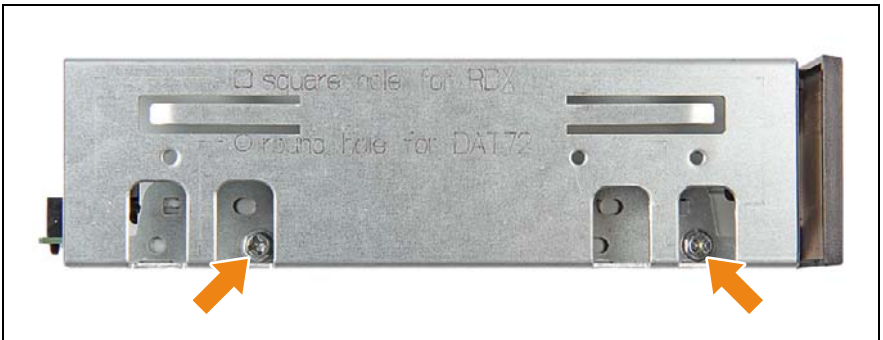
Figure 194: Securing mounting brackets to a DAT72 backup drive
