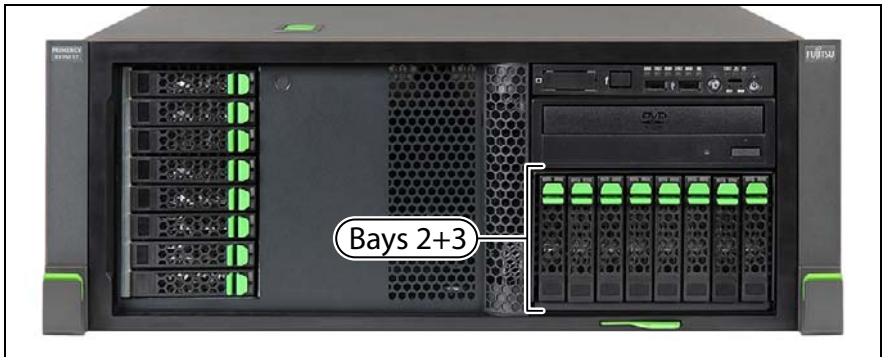
Figure 97: 8x 2.5-inch HDD extension box - Rack version
