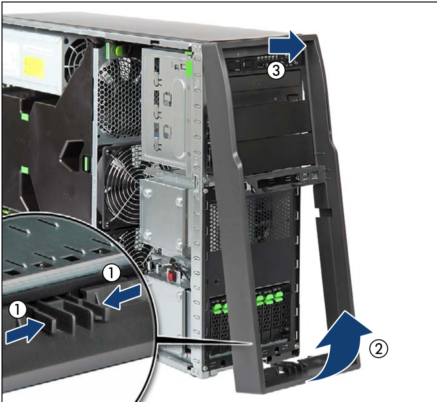
Figure 15: Removing the front cover (tower server)
