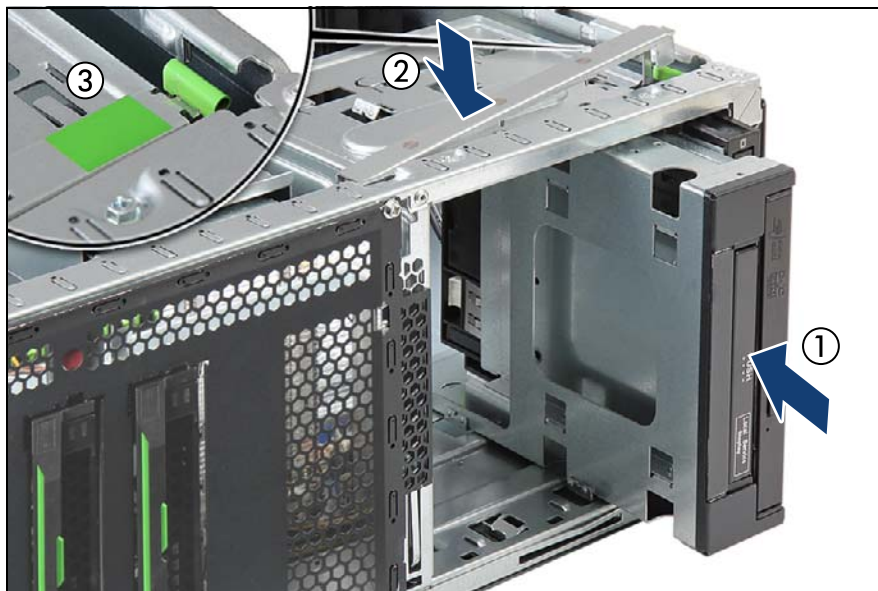
Figure 207: Inserting the Multibay box
