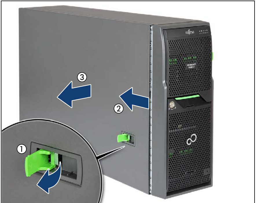
Figure 11: Removing the side cover (tower server)
