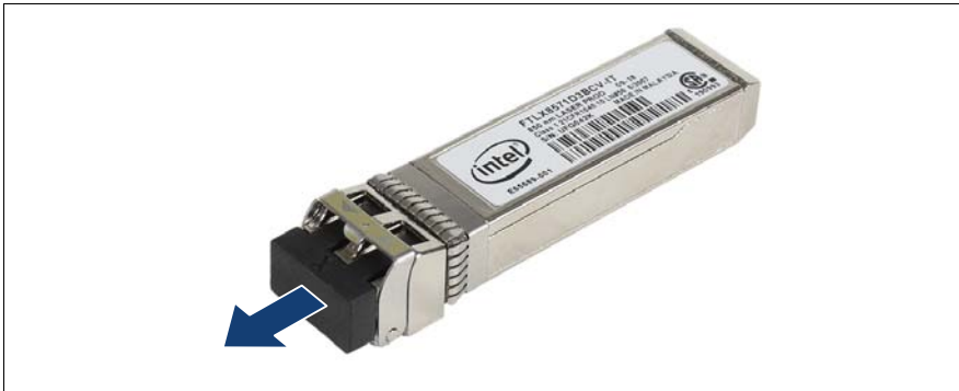
Figure 130: Removing the protective optical port plug
