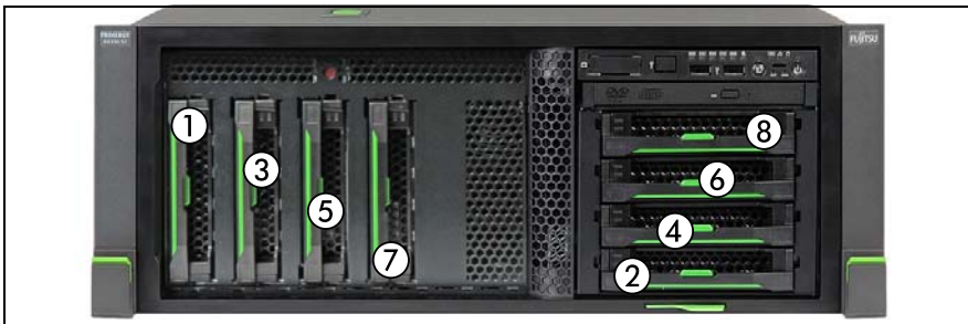
Figure 80: Mounting order with up to 8 3.5-inch HDDs (2 SAS backplanes) - Rack version
