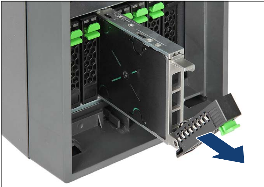
Figure 70: Removing a 2.5-inch HDD / SSD module
