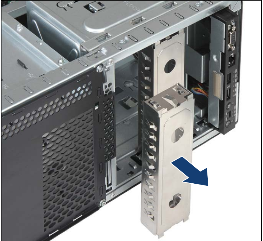
Figure 103: Removing an accessible drive filler cover
