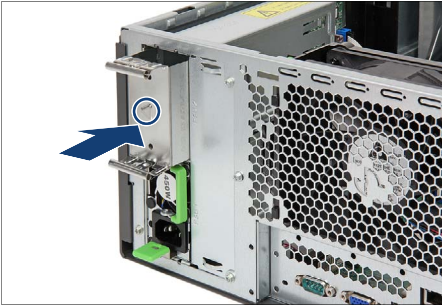
Figure 52: Installing a PSU dummy cover
