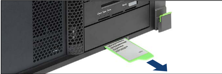
Figure 6: Removing the ID card (rack server)
