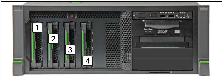
Figure 76: Naming scheme with 4 3.5-inch HDDs (1 SAS backplane)
