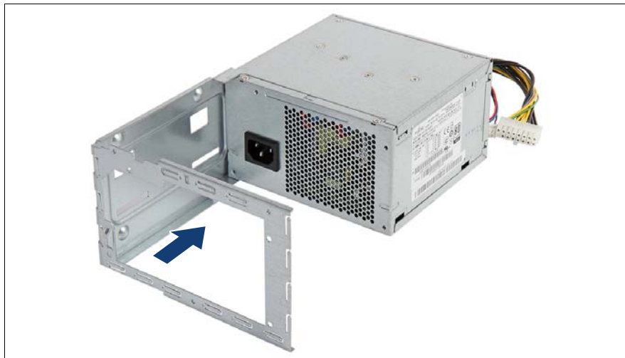
Figure 44: Installing PSU in the installation frame (A)
