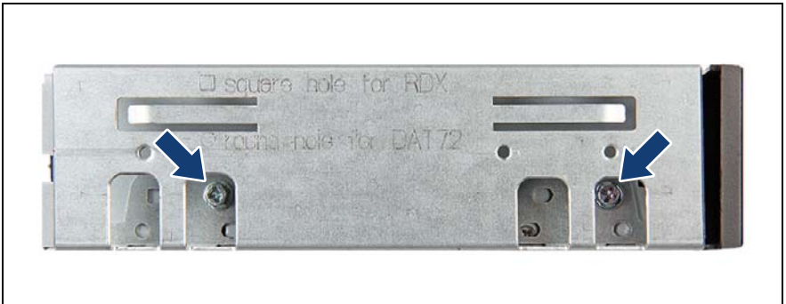
Figure 193: Securing mounting brackets to an RDX backup drive
