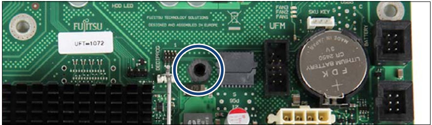
Figure 268: Removing the UFM (B)
