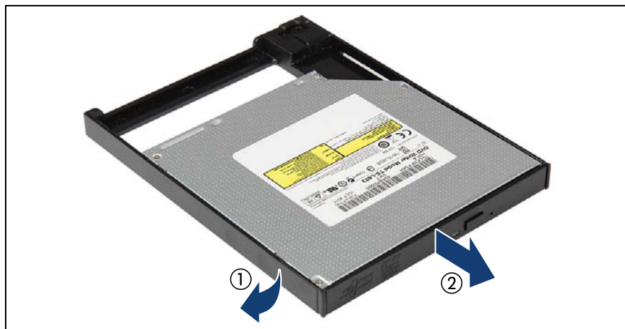
Figure 226: Removing the slimline ODD from its installation frame
