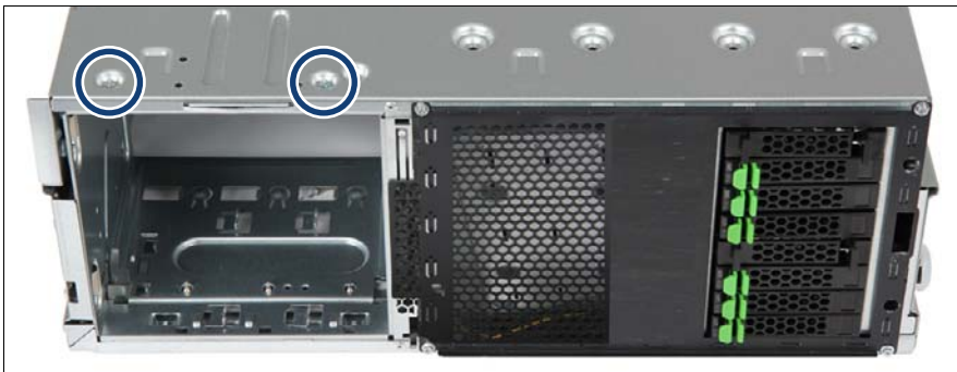
Figure 303: Securing the accessible drive cage (B)
