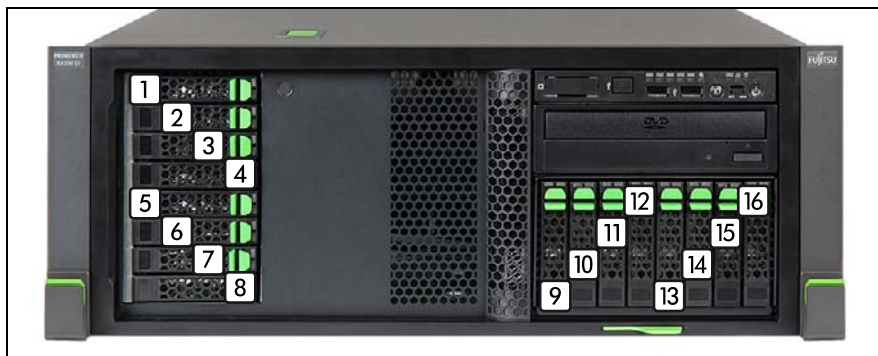
Figure 66: Naming scheme with 16 2.5-inch HDDs (4 SAS backplanes)
