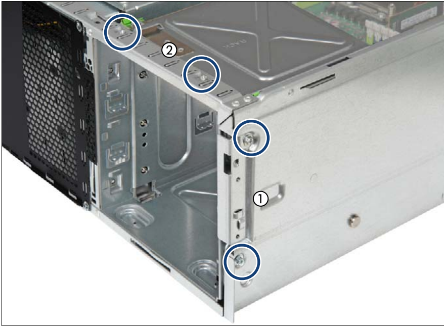
Figure 302: Securing the accessible drive cage (A)
