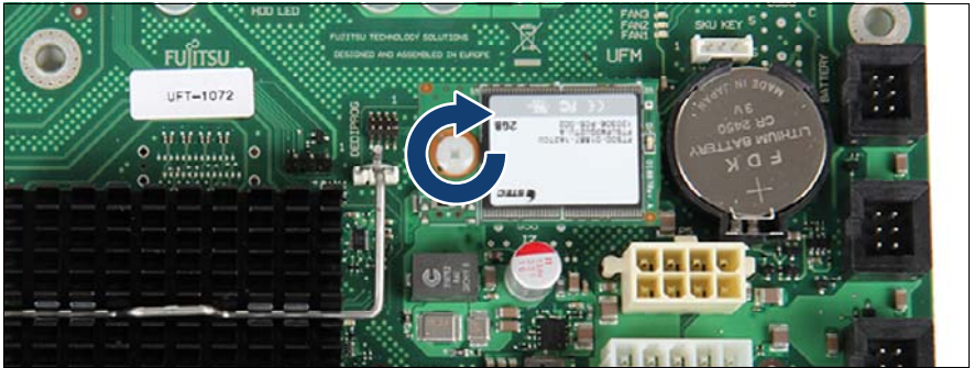
Figure 271: Installing the UFM (B)
