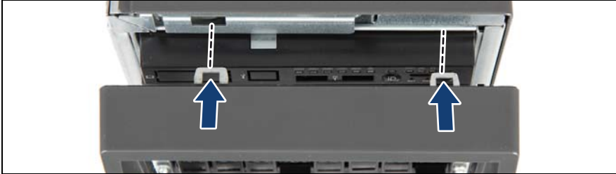
Figure 22: Installing the front cover (tower server) (A)
