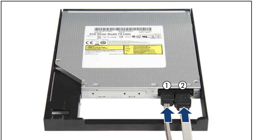
Figure 203: Mounting the slimline ODD in the installation frame (B)
