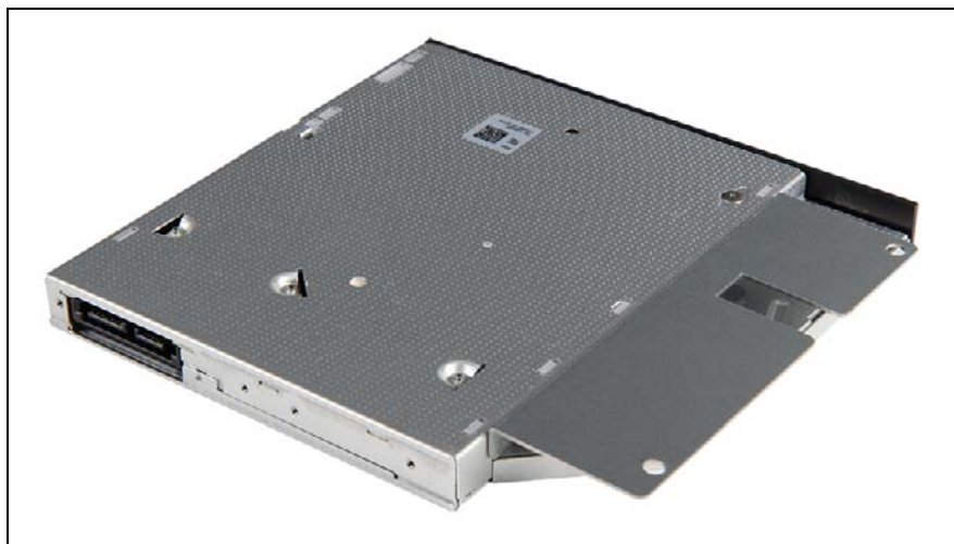
Figure 234: Installing the slimline ODD mounting bracket on the ODD (B)
