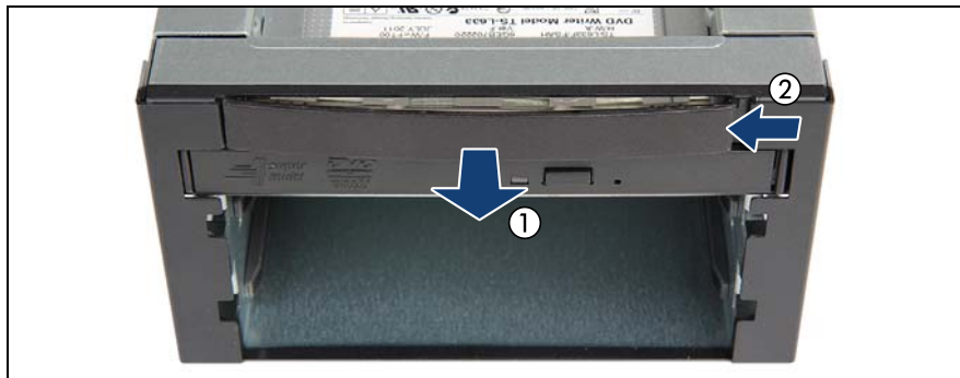
Figure 221: Removing the LSD dummy cover plate (A)
