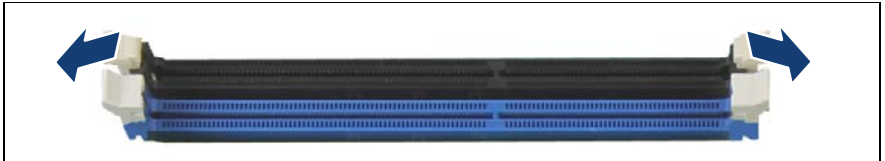
Figure 166: Installing memory modules (A)
