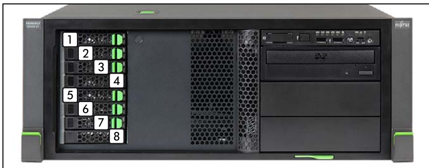
Figure 63: Naming scheme with 8 2.5-inch HDDs (2 SAS backplanes)
