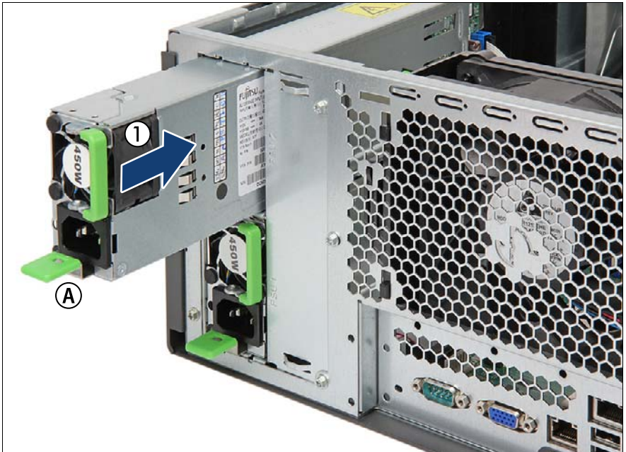
Figure 50: Installing a hot-plug PSU
