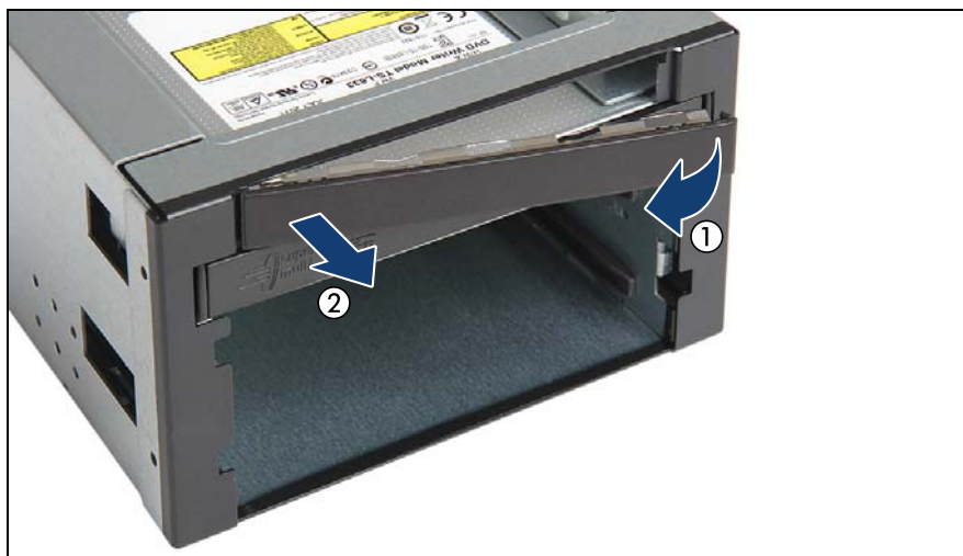
Figure 222: Removing the LSD dummy cover plate (B)
