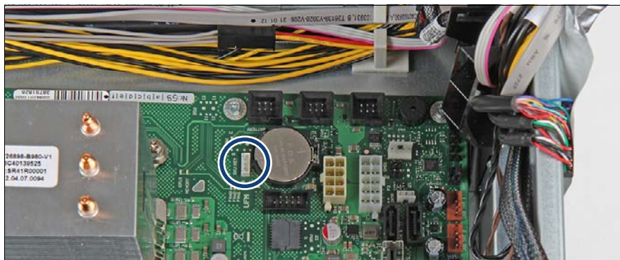
Figure 282: SCU (SKU) key mounting location
