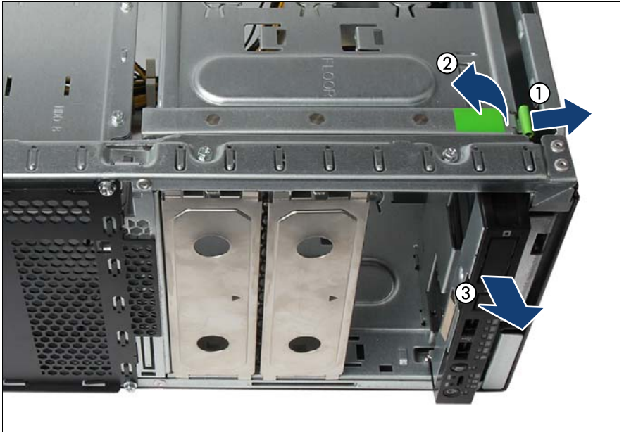
Figure 246: Removing the front panel module
