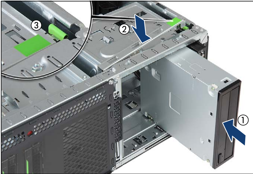
Figure 198: Inserting the accessible drive
