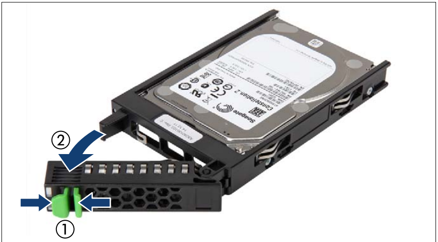
Figure 68: Opening the 2.5-inch HDD / SSD module locking lever
