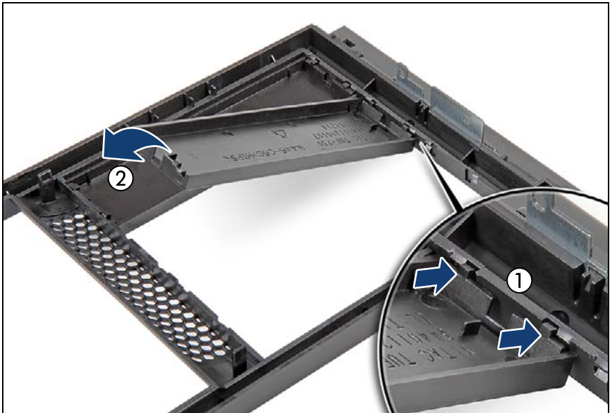
Figure 306: Installing accessible drive dummy covers
