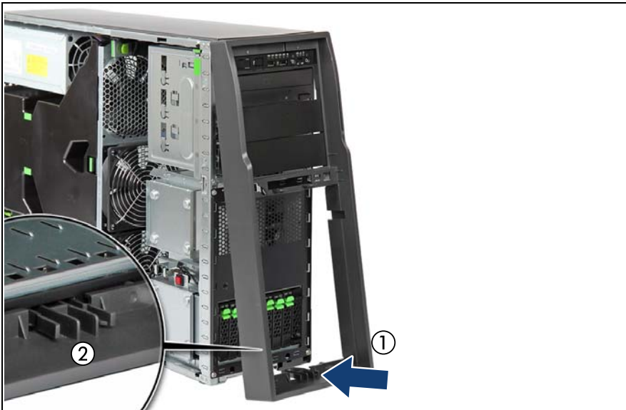
Figure 23: Installing the front cover (tower server) (B)
