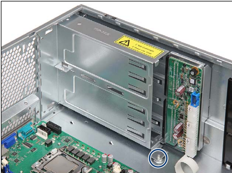
Figure 56: Securing the PSU cage (A)
