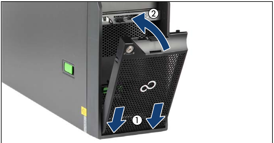
Figure 25: Installing the HDD bay cover
