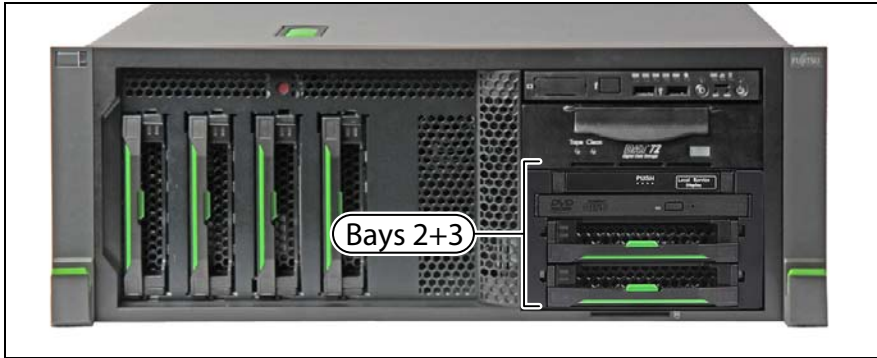
Figure 99: 2x 3.5-inch HDD extension box - Rack version
