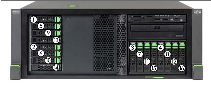
Figure 64: Mounting order with up to 16 2.5-inch HDDs (4 SAS backplanes) - Rack version
