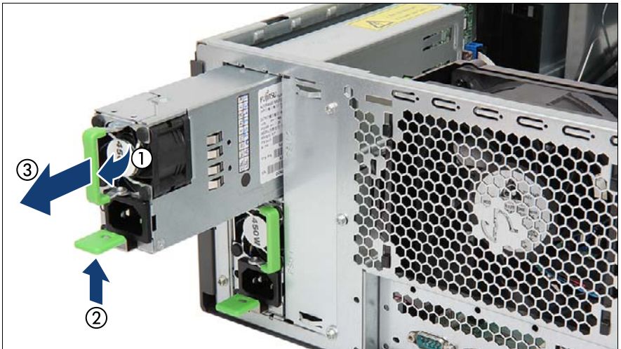
Figure 51: Removing a hot-plug PSU
