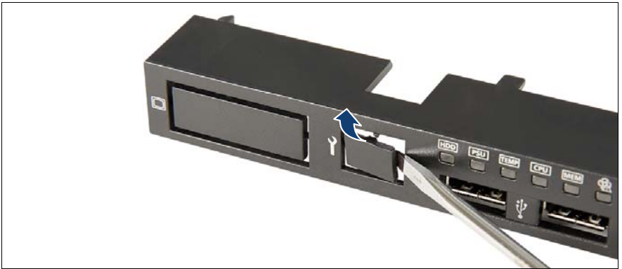
Figure 257: Breaking out the front LAN cover plate
