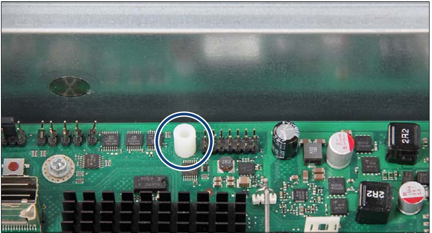
Figure 275: Installing the TPM spacer
