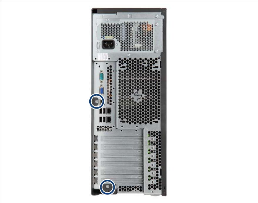
Figure 294: Removing the right side cover (A)
