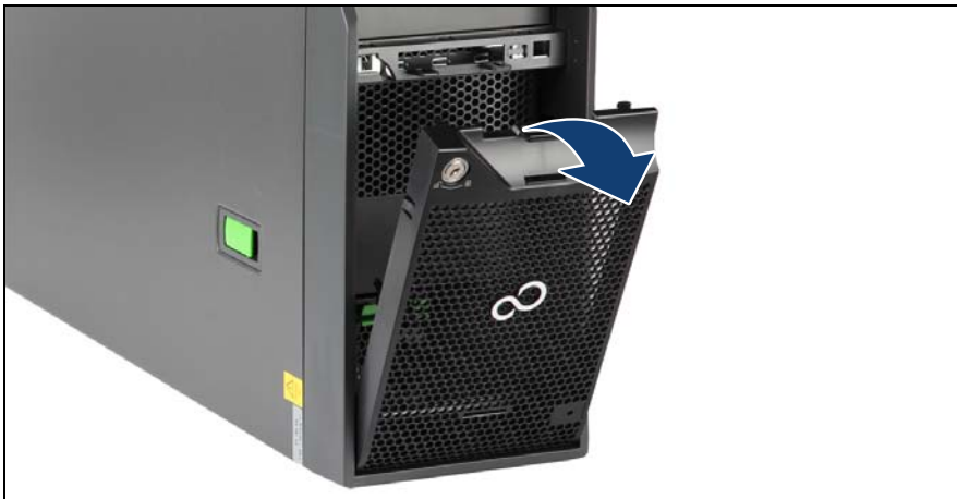
Figure 13: Removing the HDD bay cover
