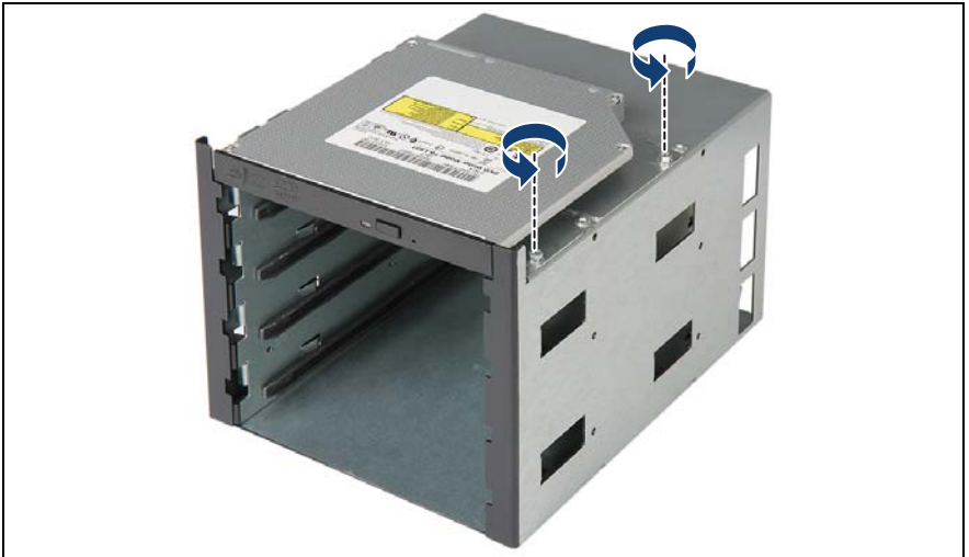
Figure 239: Removing the slimline ODD from the extension box (A)
