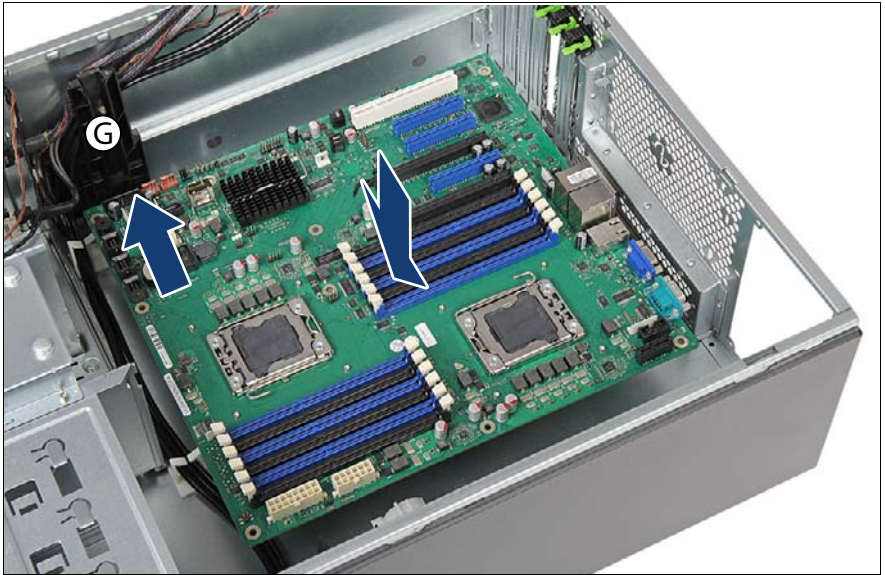
Figure 288: Installing the system board (A)
