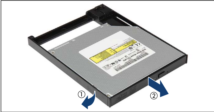
Figure 211: Removing the slimline ODD from its installation frame
