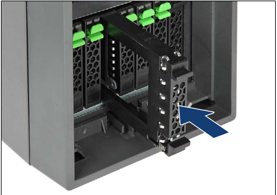
Figure 71: Installing a 2.5-inch HDD / SSD dummy module
