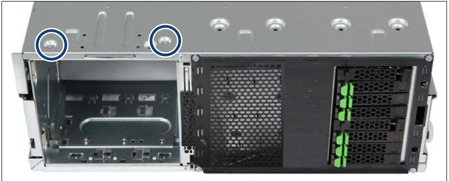
Figure 297: Detaching the accessible drive cage (A)
