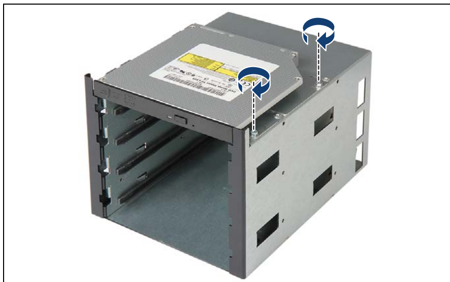
Figure 236: Installing the slimline ODD on the HDD extension box (B)
