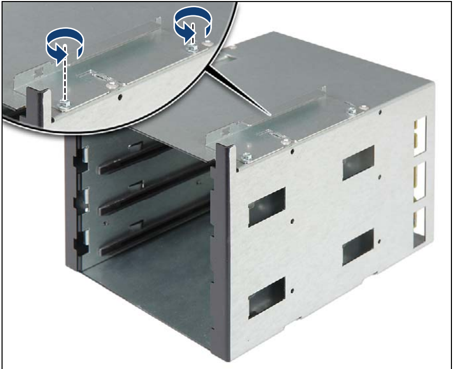
Figure 232: Removing the slimline ODD mounting bracket
