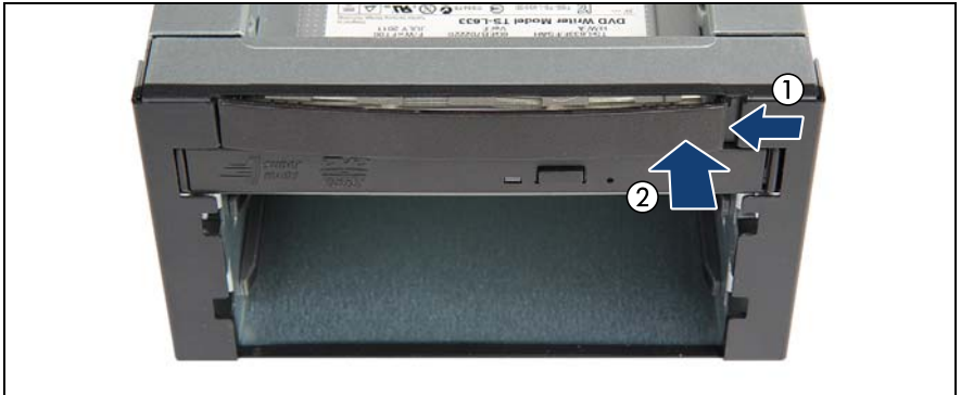
Figure 231: Mounting the slimline ODD dummy insert in the installation frame
