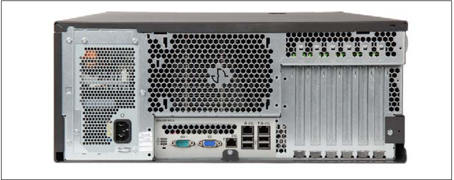
Figure 35: Server with standard PSU
