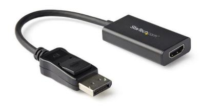
This DisplayPort to HDMI Adapter lets you connect your DP equipped computer to an HDMI display. The adapter supports High Dynamic Range (HDR) and provides sharper images with enhanced video.
