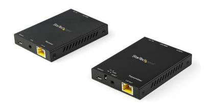
This HDMI over CAT6 extender lets you transmit your 4K 60Hz signal up to 165 ft. (50 m) over a single CAT6 cable, with the added benefit of a local HDMI output. The extender supports High Dynamic Range (HDR), providing high contrast images with enhanced video.
