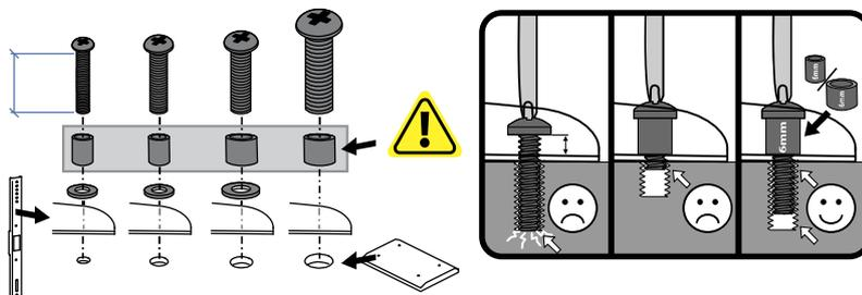
**IMPORTANT:** To ensure screws have the minimum thread engagement in the display, tighten screws with at least six, full, 360° revolutions.
