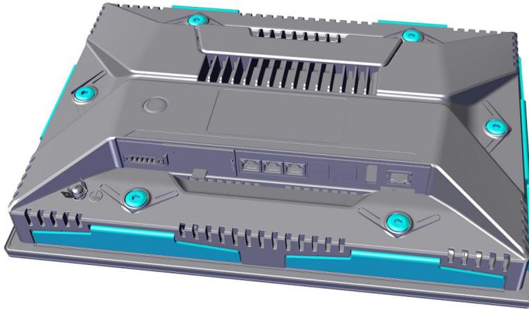
5. Make sure that all clamps are fully in contact with the rear side of the recess.
