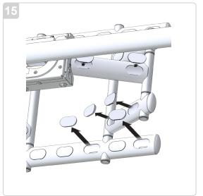
Once all mounting points and level of the display have been confirmed, remove the plastic covers to route cable from the wall to the display.
