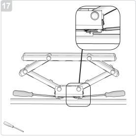
The two side mounted screws in the receiver head of the mount can be adjusted to add or subtract tension in the rotation of the display in the mount.
