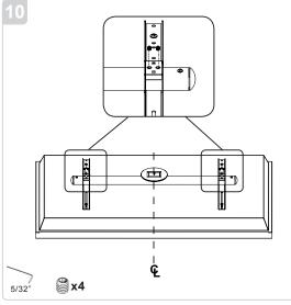
Invert the flat panel display and place it on a smooth flat surface so the back of the display panel is facing up. Align the two mounting bracket to the four mounting points on the rear of the display and secure them bracket to the display with the proper "pitch" supplied hardware. Check the owners manual to determine correct pitch hardware recommended.
