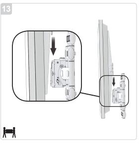
Note: appropriate number of personal and possible installation lift aids lift and insert the round portion of the crossbar with display attached and safely insert the round portion of the cross bar into the open round receiver portion on the wall mount.
