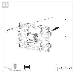
With minimum two people place the PFW 6855 wall plate assembly and secure to the wall using the top center hole of the wall plate.
