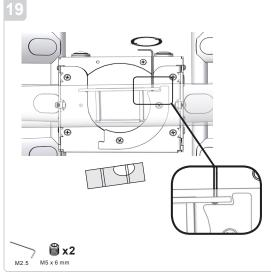
With the 2.5mm Allen head wrench supplied, install the two each M5 x 6mm mini adjustment Allen head screws supplied to both sides of the "rotation" stop bar. Slowly turn the display to the level position in each direction and adjust the two adjust screw to set max rotation in each direction to level.
