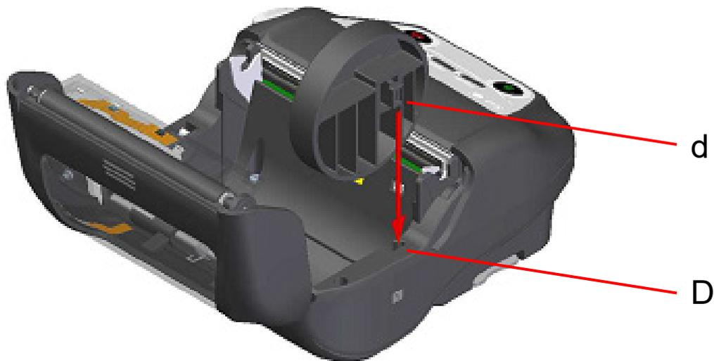
Figure 14-1 Installing Partition Plate (1)
