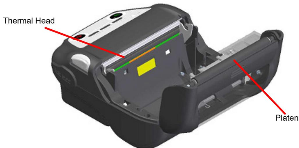
**Figure 20-1 Cleaning Thermal Head / Platen**
