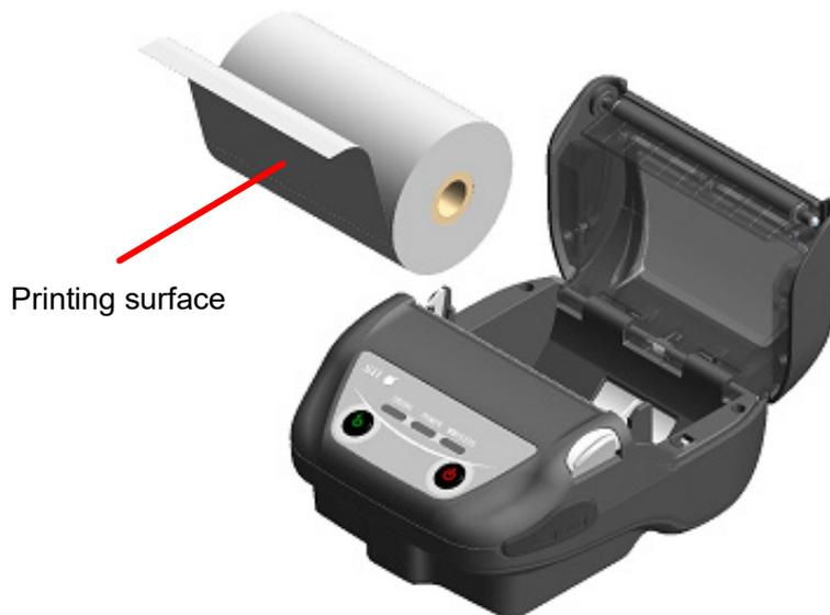
**Figure 9-2 Thermal Paper Setting Direction**
