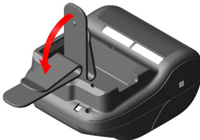
Figure 15-2 Installing Belt Clip (2)
