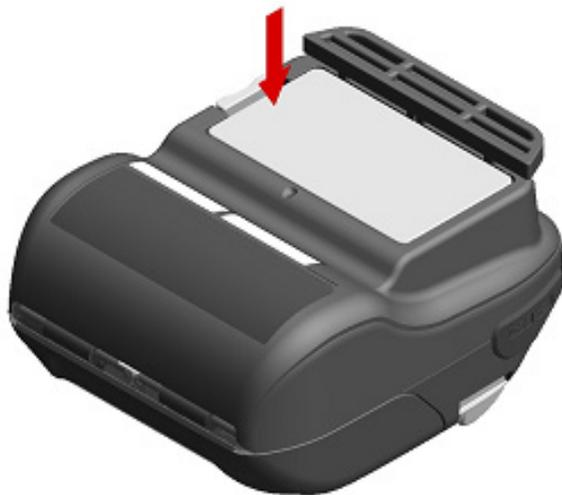
**Figure 15-6** Installing Shoulder Strap (2)
