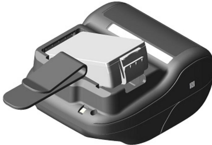
**Figure 15-3 Installing Belt Clip (3)**
