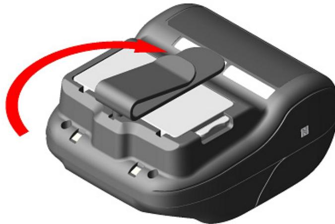
**Figure 15-4 Installing Belt Clip (4)**
