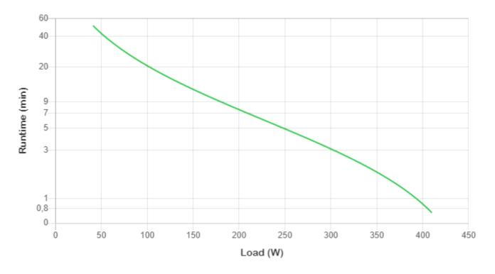
Curve fit to measured runtime data. All measurements taken with new, fully charged batteries, at typical environmental conditions, with no electrical input and balanced resistive load (PF = 1.0) output.
