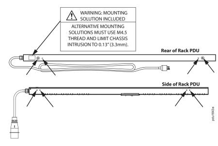
Two Rack PDUs can be installed on one vertical accessory channel in a NetShelter rack.
