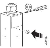
NOTE: The installation's receptacle/socket-outlet must have a Protective Earthing Connection. The plug on the power supply cord connects the Rack PDU's Protective Earthing Conductor to the installation's Protective Earthing Conductor.
