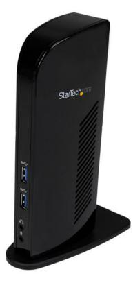
The USB3SDOCKHD Universal USB 3.0 Laptop Docking Station with DVI, HDMI, Audio and Ethernet adds dual video outputs, headphone and microphone jacks, as well as Gigabit Ethernet and additional USB 3.0 and USB 2.0 ports to a laptop computer, all from a single device and over a single SuperSpeed USB 3.0 connection.
