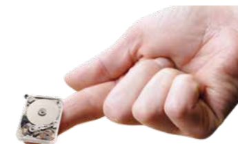
The mini-disk measures exactly 0.85 inches – about the size of a one euro coin, and almost as flat.
