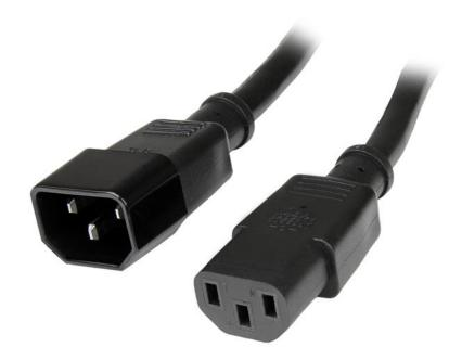
The PXT1001M 1m PDU Style Computer Power Extension Cord features one C13 computer power (female) connector and one C14 hooded (male) power connector, and enables you to connect your server to a C13-equipped UPS or PDU.
