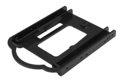
This mounting bracket lets you quickly install a 2.5" SSD or HDD into a single 3.5" bay in a desktop PC or server, with no tools required. The tool-less mounting bracket supports a 2.5" solid-state drive or hard drive from 7 mm to 9.5 mm in height.
