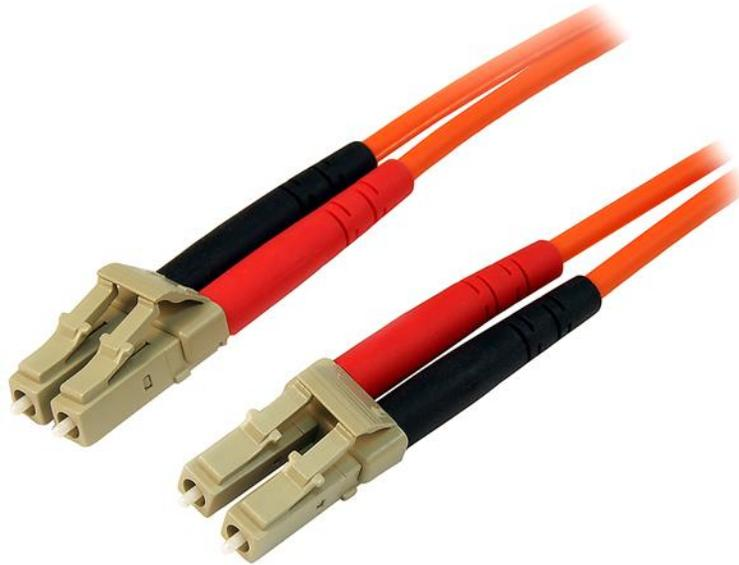
The 50FIBLCLC1 1m LSZH LC to LC Fiber Cable features 50/125 micron fiber for high-speed, high bandwidth data transmissions over Gigabit Ethernet and Fiber Channel networks, with support for duplex multimode applications.
