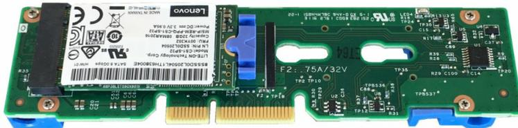
Figure 13. ThinkSystem M.2 Enablement Kit (shown with a 32 GB M.2 drive, not supported in the SE350)
