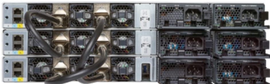
Figure 5. Cisco Catalyst 9300 Series switch stack units
