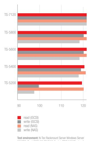
**Test environment:** N-Tec Rackmount Server Windows Server 2008R2, Dual XEON 32 GB RAM, 2 x IntelPRO/1000Dual = 4 x Gigabit NIC; Cisco SG300-10P 10 Port managed Gigabit with PoE.
