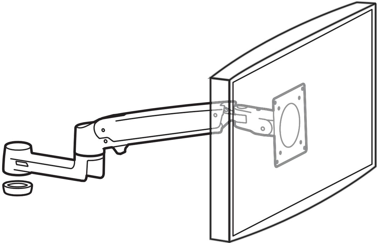
**⚠ CAUTION!** The LX Arm Accessory is designed to be used with the 45-295 LX Desk Mount LCD Arm, Tall Pole and the 45-509 LX Dual Stacking Arm, Tall pole products. Using the LX Arm Accessory with any other product may create an unstable situation resulting in equipment damage and/or personal injury.
