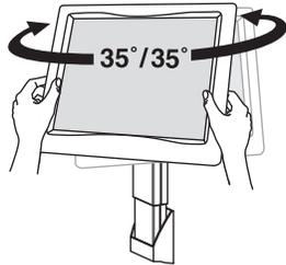
LCD tilts forward/back up to 35°\*
