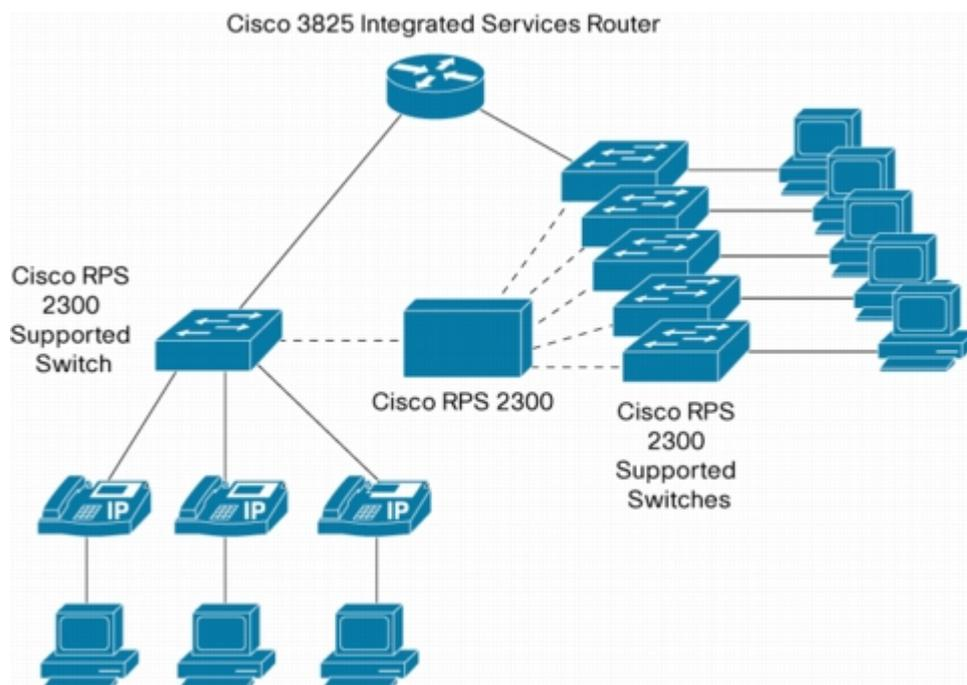
When designing or upgrading a wiring closet, careful consideration should be given to power requirements, particularly for PoE deployments. A power architecture can be selected based on the level of availability desired. The primary power faults to protect against include:
