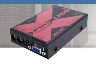
Second generation extender to transmit VGA video, audio and transparent USB over CATx cable
