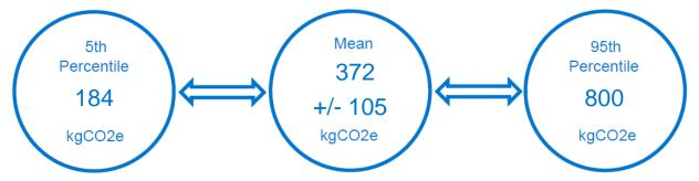
Carbon footprint calculations have a wide range based on a variety of factors including how the device is configured, where it was manufactured and more. Dell Technologies reports the 5th and 95th percentile of the carbon footprint estimate to reflect that uncertainty. For this product, that estimate has a mean of 372 kg of CO2e and standard deviation of 105 kg of CO2e.
