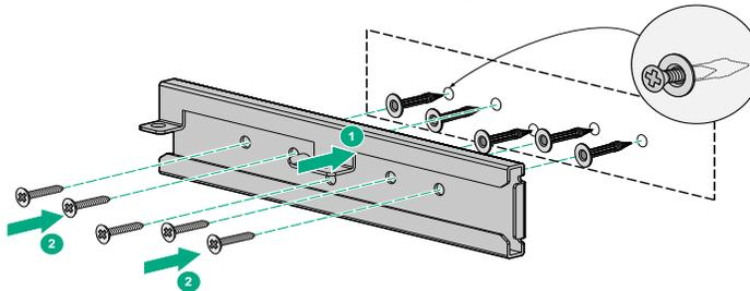
3. Connect the two mount brackets by bringing in the bracket without the plastic rivet at an angle and clicking it into place, making sure the hemmed edges are facing the same way (see Figure 2).
