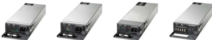
Figure 2. Redundant Power Supplies
