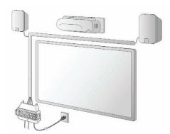
Speakers, projector and Control Box typical installation.
