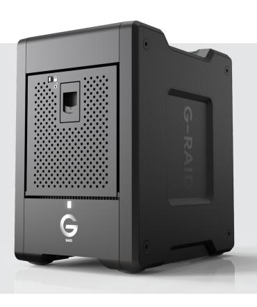
A transportable 8-bay hardware RAID solution, the G-RAID™ SHUTTLE SSD with Thunderbolt™ 3 (40Gbps) and USB-C™ (10Gbps) interfaces offers professionals up to 32TB¹ of massive capacity and high-powered performance for super-fast access, and real-time video editing. Supports multi-stream 4K, 8K, and VR workflows, RAID 0, 1, 5, 10, and 50 configurations, and provides turbocharged transfer rates up to 2800MB/s read and 2700MB/s write.²
