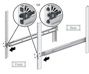
1. Fully extend the inner rail outwards until you hear a click sound. 2. Pull and hold the rear latch on the inner rail, as illustrated,  $% \left( 1\right) =\left( 1\right) \left( 1\right)$ and continue to pull out the inner rail from the assembly.
