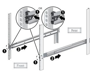
Pull the rear latch of the inner rail assembly, and slide forwards to remove the assembly from the rack.
