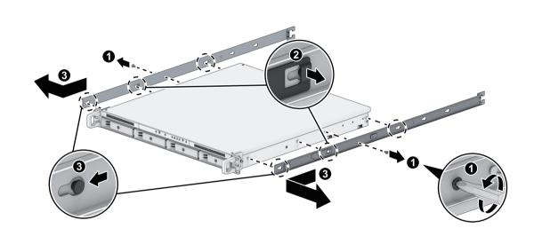
$05 \quad \text{Insert the inner rail to the rail kit assembly by pulling outwards} \\ \text{and holding its front latch.}$
