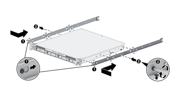
With the help of another person, carefully align the inner rails to the outer rail assembly, and push the chassis towards the rack.
