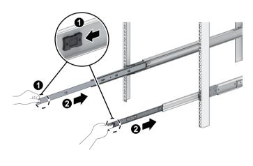
Push the front latch of the inner rail assembly, and slide backwards to remove the assembly from the rack.
