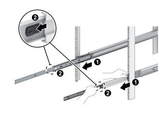
1. Align the fixing holes of the inner rail to the side of the chassis and slide backward to attach the inner rail. 2. Secure the inner rail screws as illustrated.
