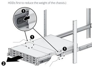
Loosen and remove the rail screws. Slightly pull out the middle latch as illustrated, and slide forwards to remove the inner rail from the chassis.
