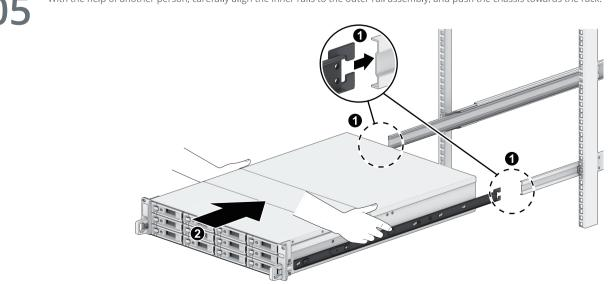
inner rail, and continue pushing the chassis towards the rack.
