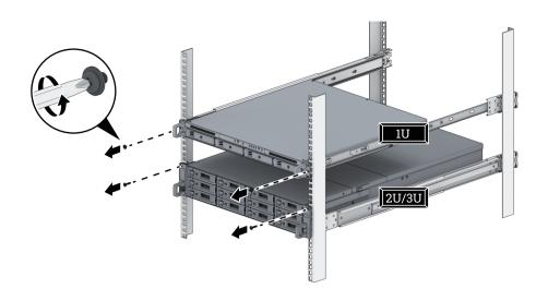
For 2U/3U chassis, slide inwards and hold the rail kit release tabs on the ear holders, and pull out the chassis from the rack.
