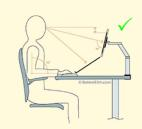
The Filex Galaxy Modular Dual is an ideal monitor arm for your workspace layout. The monitor arm has a gas spring technology that makes it easy to quickly set the screen to any desired height. An optimal monitor position causes fewer neck problems (Kumar 1994 McKinnon 1994, Marcus 2002). Placing the monitor too low can make you bend your neck excessively and strain your neck muscles. An optimal screen height increases productivity by 10% (Sommerich et al., 1998).
