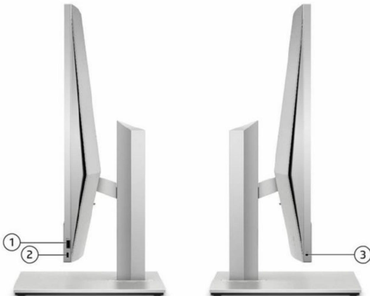
1. Type-A SuperSpeed USB 10Gbps signaling rate port (charge support up to 5V/3A)
