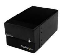
The S3520BU33ER 2-Bay RAID Enclosure offers a high-performance external storage solution, enabling you to build a secure RAID array with two 3.5" SATA hard drives, with the option to connect it to your computer through either an available USB 3.0 or eSATA port.
