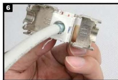
Install the termination cap in direction of arrow into the Keystone Jack.
