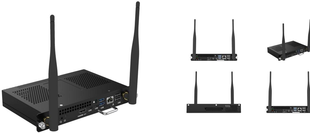
**An Intel® i5 OPS slot PC with Windows® 11 which supports 5K (5120x2160) resolution**
