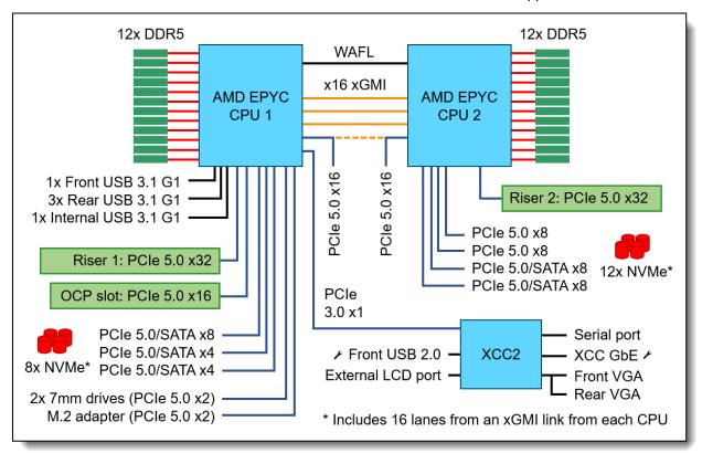
Figure 5. SR665 V3 system architectural block diagram
