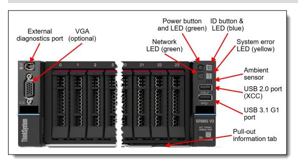
Figure 20. Front operator controls are on the left and right side of the server
