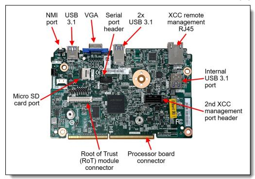
Figure 19. System I/O Board
