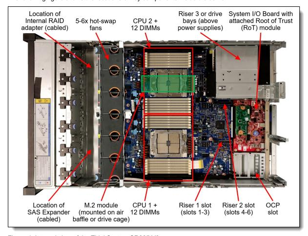
Figure 4. Internal view of the ThinkSystem SR665 V3
