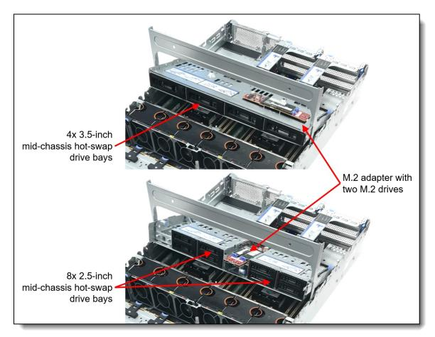
Figure 10. Mid-chassis drive bays
