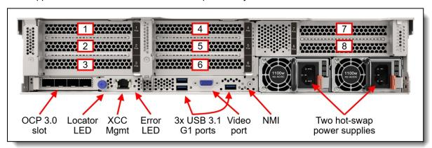
Figure 3. Rear view of the ThinkSystem SR665 V3 (configuration with eight full-height PCIe slots) The following figure shows the locations of key components inside the server.
