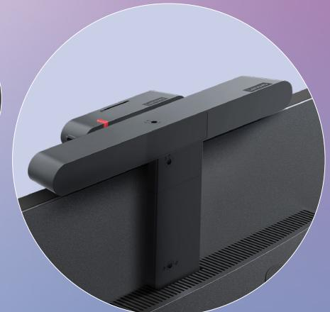
Visual representation of VoIP Stack after being mounted on the monitor
