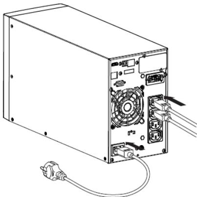
1-Connect the UPS input socket to the AC-power source using the cable of the protected equipment.
