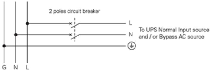
**Input terminal and output terminal connection:**
