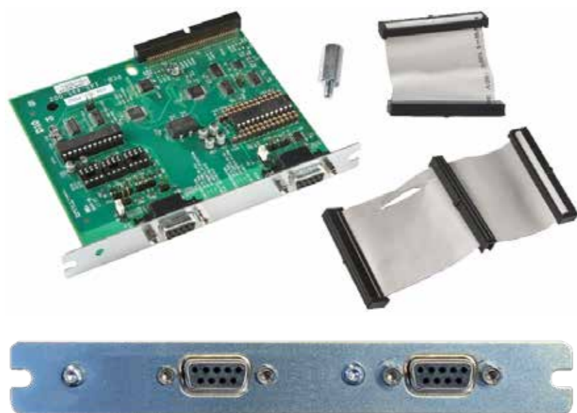
PX45 / PX65 has 2 x I/O Expansion Slots
