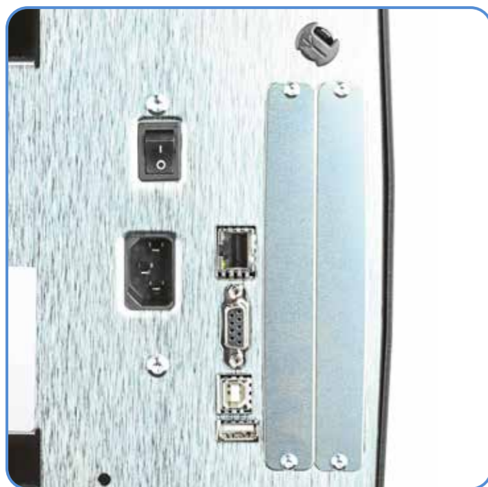
PX45 / PX65 has 2 x I/O Expansion Slots
