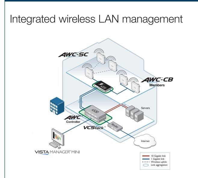
Allied Telesis Autonomous Wave Controller (AWC) offers solutions for two of the most common problems with Wireless LANs: initial setup complexity and on-going performance degradation. Initial WLAN set-up usually requires a site survey to achieve the best coverage; and performance of WLANs can often change over time as external sources of radio interference reduce coverage and bandwidth. These issues can be time-consuming to identify and resolve.
