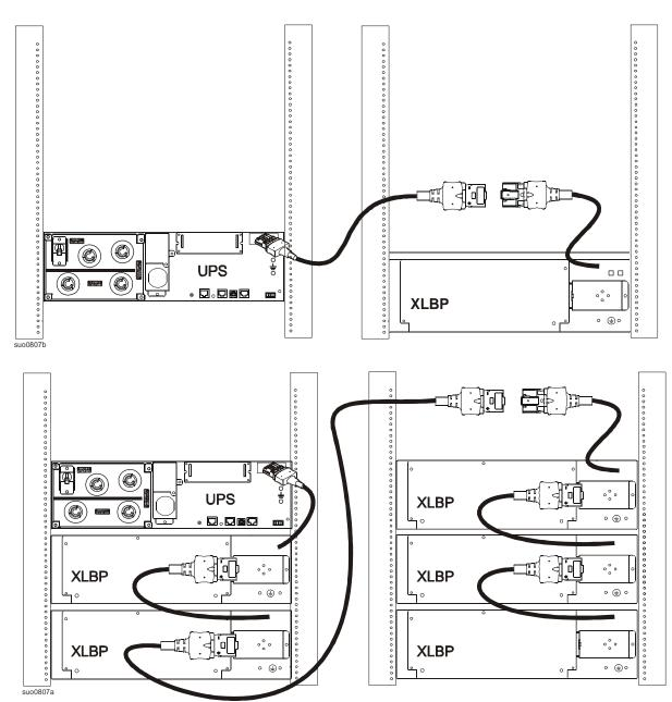
One UPS and one external battery pack with external battery pack extension cable connection.
