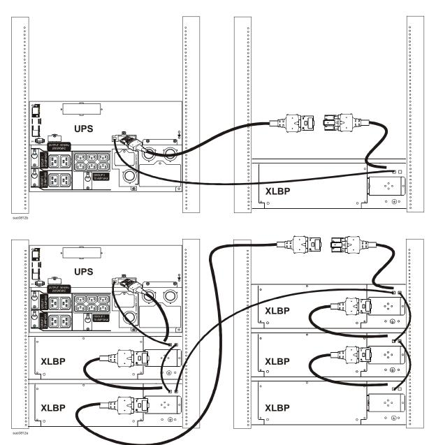
One UPS and one external battery pack with communication cable connection and external battery pack extension cable connection.
