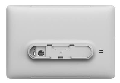
Above: The I/O section of Cisco Room Navigator for Table with the foot stand deattached from the touch panel.
