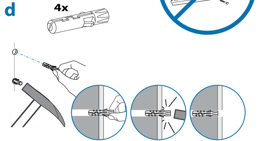
**WARNING:** Mounting holes must be at least 3-1/8" (80mm) deep and must be located within solid concrete, not mortar or covering material. If you drill into an area of concrete that is not solid, reposition mounting holes until both anchors can be fully inserted into solid concrete!
