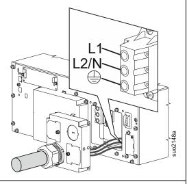
Install the hardwire terminal cover removed in step 3.
