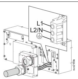
Insert the output wire through the strain relief and secure the wires to the output terminals.
