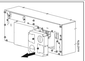
Install the snap-in strain reliefs (supplied) in both the input and output knock-outs.
