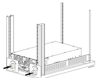
Rotate the BATTERY ON/OFF switch in counter clockwise direction to turn on the battery pack.
