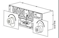
To slide out the left battery module push down and hold the thumbscrew and slide out the battery module.
