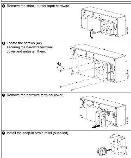
Insert the input wire through the strain relief and secure the wires to the input terminals.
