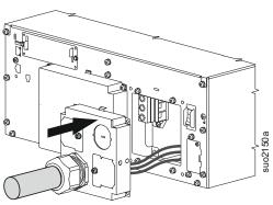
Secure the hardwire terminal cover by fastening the screws (4x).
