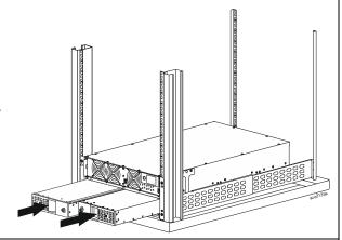
Press the thumbscrew (in each battery module) till it engages and turn the thumbscrew clockwise to lock the battery and enable battery communication.
