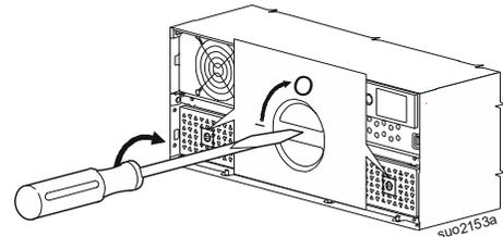
**3** Turn the thumbscrew counter clockwise to unlock the battery module.
