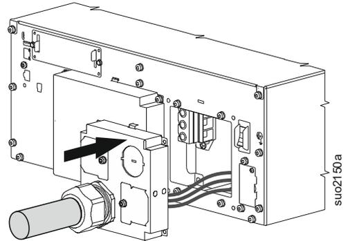
7 Secure the hardwire terminal cover by fastening the screws (4x).
