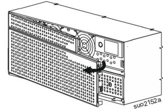
**2** Turn the BATTERY ON/OFF switch in clockwise direction (applicable to both left and right battery modules), using a screwdriver, to switch *off* the battery.
