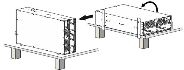
3 Slide the battery pack till it gets fully inserted into the UPS.
