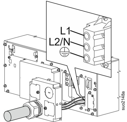
6 Install the hardwire terminal cover removed in step 3.
