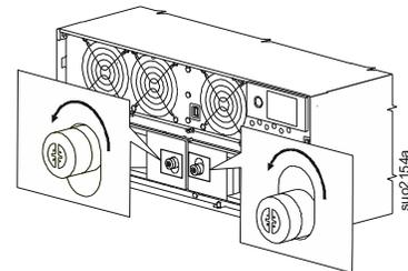
**4** To slide out the left battery module push down and hold the thumbscrew and slide out the battery module.
