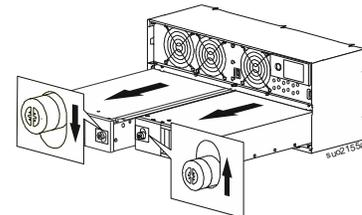
**5** Slide the replacement battery module into the UPS till it gets locked in position.
